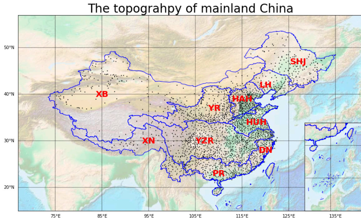
Figure 1. High-density rain gauge observation network (black dots) and main hydrological basins in China (blue outline). Base map is the topography of mainland China (Map Registration No. GS (2016)2885). The lower-right subplot displays the South China Sea. The 10 sub regions used in this study are as follows: (a) Songhua River Basin (SHJ), (b) Liaohe River Basin (LH), (c) river basins in northwest China (XB), (d) Haihe River Basin (HAH), (e) Yellow River Basin (YR), (f) Yangtze River Basin (YZR), (g) Huaihe River Basin (HUH), (h) River Basins in Southeast China (DN), (i) river basins in southwest China (XN), and (j) Pearl River Basin (PR).
