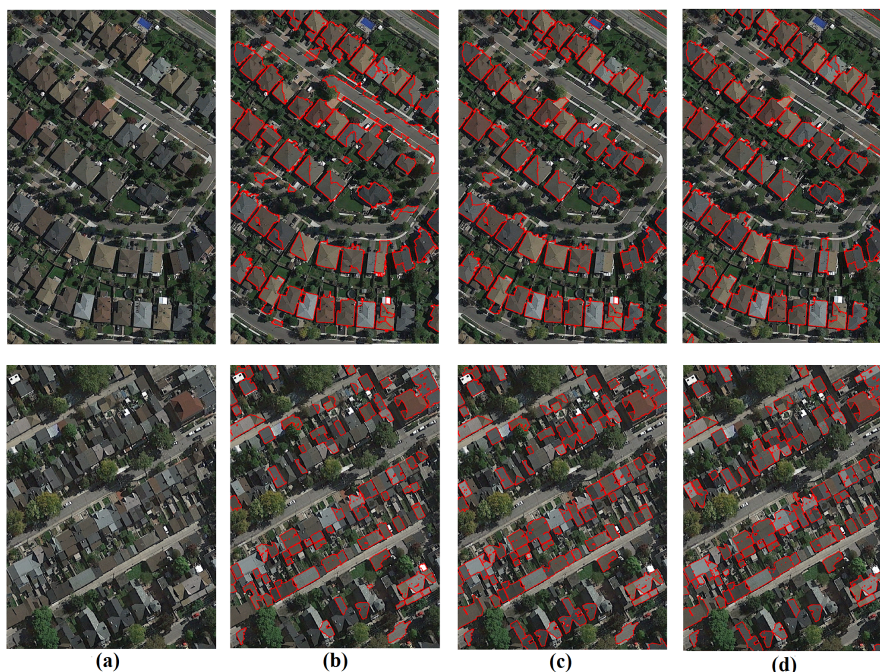
Figure 10. House detection results on image test1 (first row) and test8 (second row). (a) Original images; (b) Results of AdaBoost; (c) Results of Random Forest (RF); (d) Results of Support Vector Machine (SVM).
