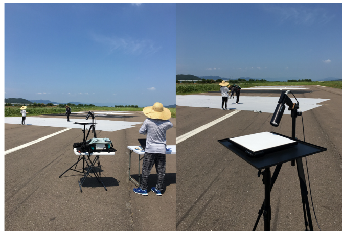
Figure 5. Picture showing radiance measurements of a white reference panel and calibration tarps using a dual ASD FieldSpec ® 3 radiometer system at Goheung site in South Korea.
