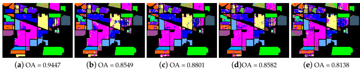
Figure 11. NN classification results on noisy Indian Pines image (noise variance \sigma = 250 ) obtained by: (a) BLRDA; (b) BSDA; (c) BKDA; (d) BLEDA; (e) IFRF.
