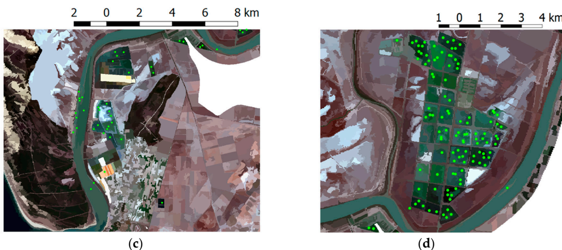
Figure 5. (a) Initial inundation map generated after applying T_{init} to the SWIR band (the centroids of the segments having a large percentage of inundated pixels are visualized as green dots) with three subsets denoted on the map; (b) additional inundated pixels found after applying T_{final} to the SWIR band, compared to the initial inundation map, for Subsets 2 and 3; (c) the mean-shift segmentation map of Subset 1 with the included centroids; and (d) the mean-shift segmentation map of Subset 2 with the included centroids.
