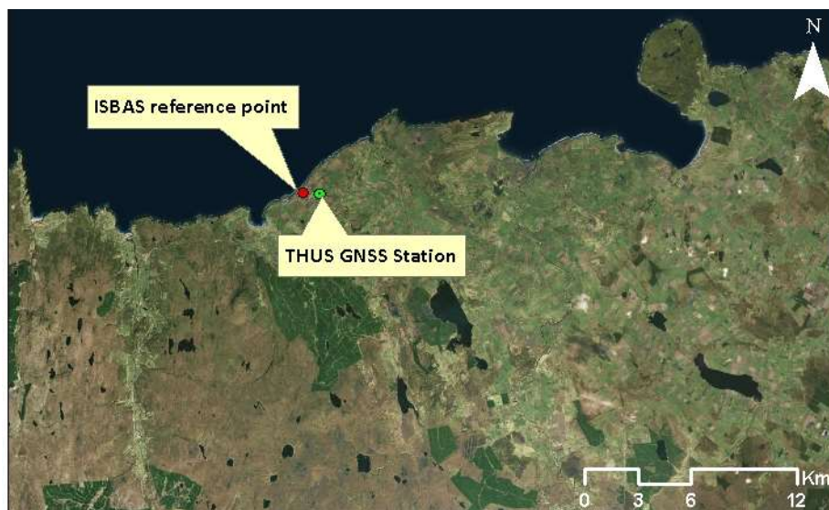
Figure 3. Relative location of ISBAS reference point used and the nearby Thurso (THUS) GNSS station: comparison of the motion data from the two indicates stability of the reference point.
