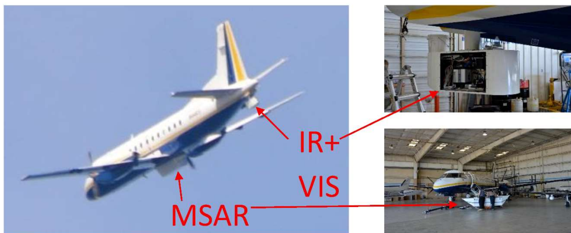
Figure 1. (left) Photograph of the remote sensing aircraft SAAB 340 with (upper right) infrared and visible sensors enclosure and (lower right) MSAR radome.
