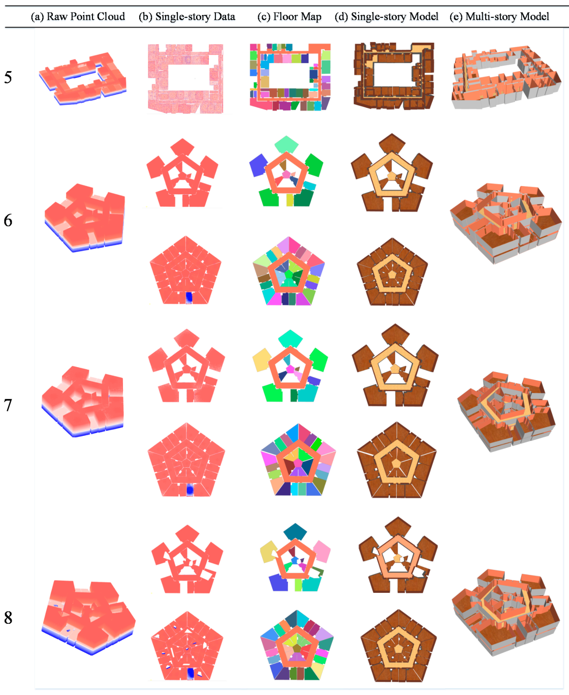
Figure 15. Synthetic data reconstruction results. (a) Original data (certain datasets have the ceilings removed for clarity). (b) Top view of data for one story. (c) Reconstructed floor map of one story. (d) Indoor-reconstruction models of one story that were colored in Google Sketchup. (e) Reconstruction of a multistory building.
