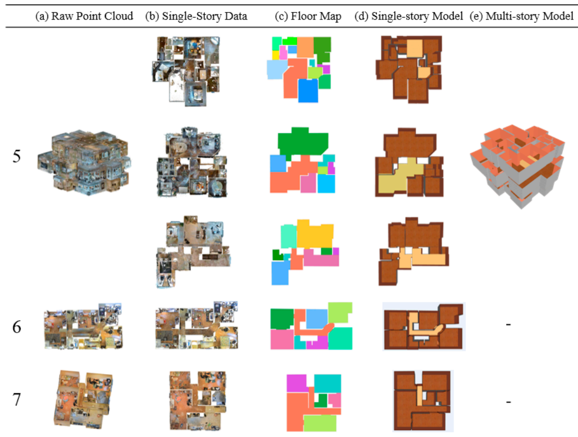
Figure 14. Results of indoor reconstruction. (a) Original data (certain datasets have the ceilings removed for clarity). (b) Top view of data for one story. (c) Reconstructed floor map of one story. (d) Indoor-reconstruction models of a single story that were colored in Google Sketchup. (e) Reconstruction of a multistory building.
