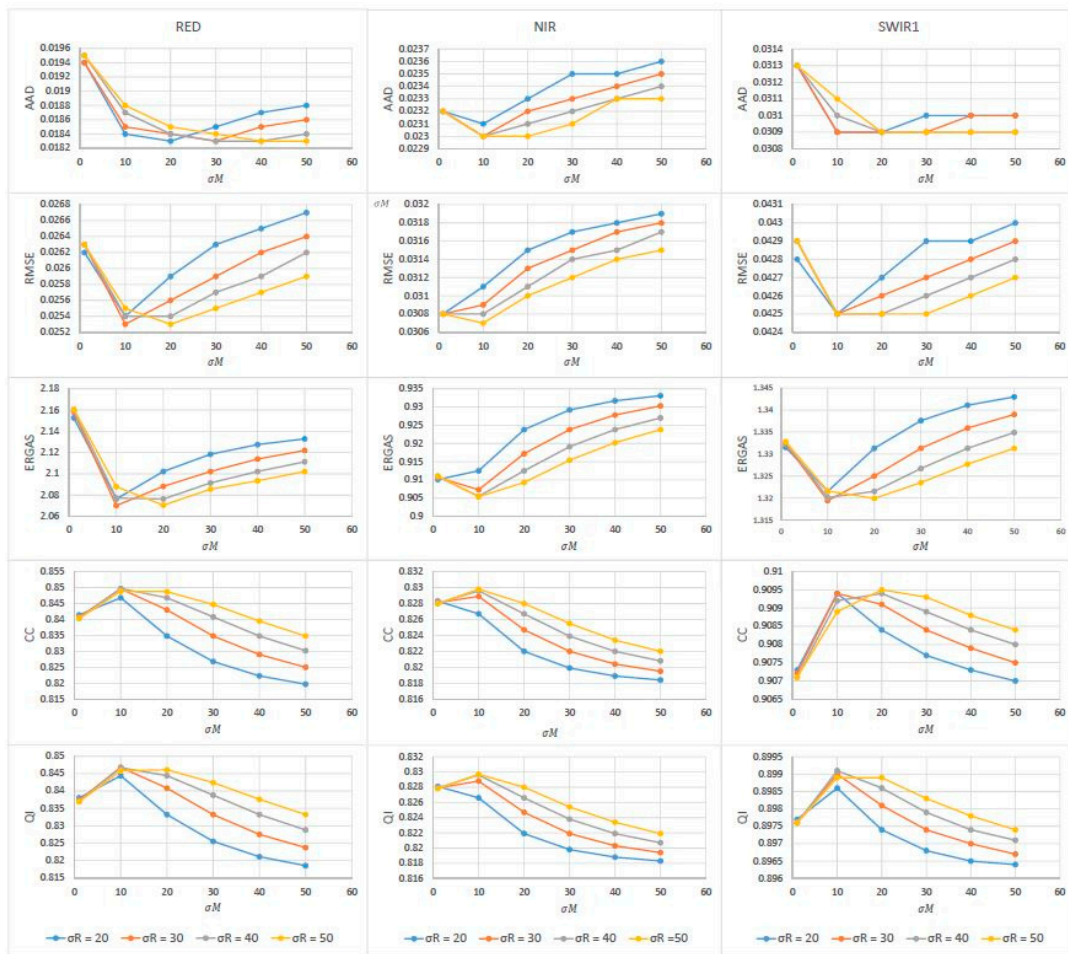
Figure 7. Quality indices comparison of the predicted Landsat-like images by PSRFM with different priori uncertainties set ranged from 20 to 50 and from 1 to 50 for the input Landsat and MODIS images, respectively. The different colors represent the priori uncertainties used for the input Landsat images \sigma_R . The graphic curves represent changes of quality indices with different priori uncertainties ( \sigma_M ) used for the input MODIS images. The columns present the three bands RED, NIR and SWIR1, respectively.
