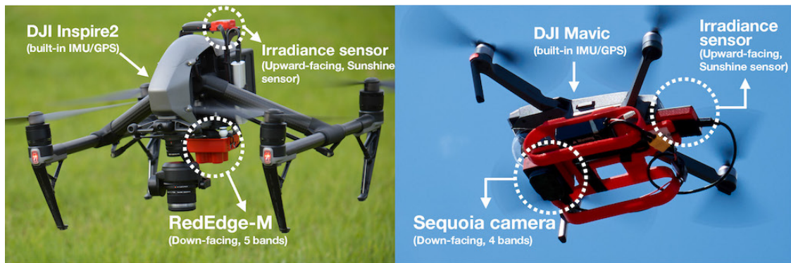
Figure 4. Multispectral cameras and irradiance (Sunshine) sensors' configuration. Both cameras are facing-down with respect to the drone body and irradiance sensors are facing-up.
