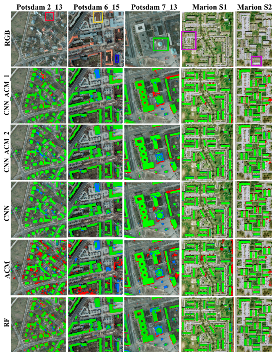
Figure 6. The detected buildings in five test scenes with five different methods. Areas in the green color denote TP , areas in the blue color denote FN , and areas in the red color denote FP at the object level.
