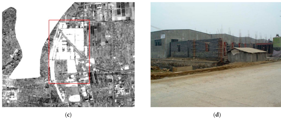
Figure 4. Example of PCA-enhanced land use change information from cropland and water to urban land in the third principal component (PC3), 2003–2006. (a) RGB composition image of SPOT-5 (2003); (b) (RGB) composition image of SPOT-5 (2006); (c) the third principal component; (d) field survey photo (2006).
