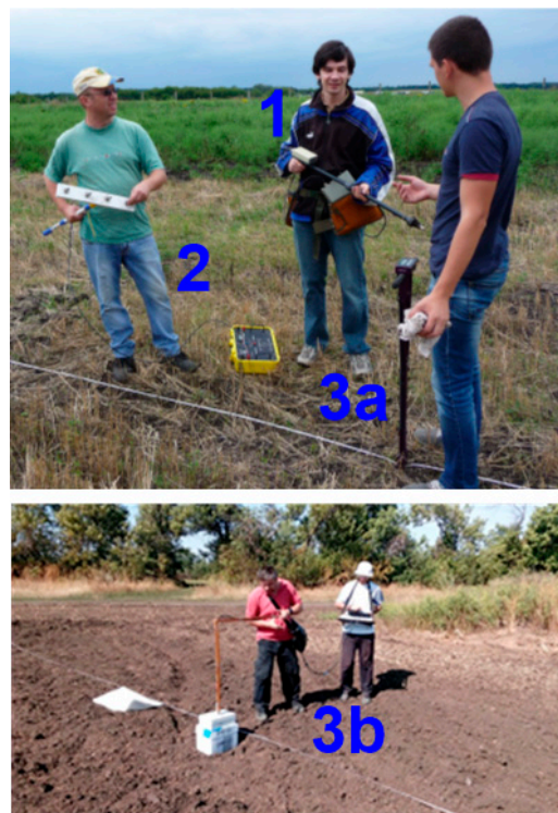
Figure 3. Photographs of field equipment. (1) Bartington MS2 magnetic susceptibility meter with MS2F probe, (2) L&R Instruments MiniRes with 4-electrode probe. (3a) Spectrum Technologies Field Scout 300 TDR. (3b) Purpose-built 1-Tx, 2-Rx impulse GPR.
