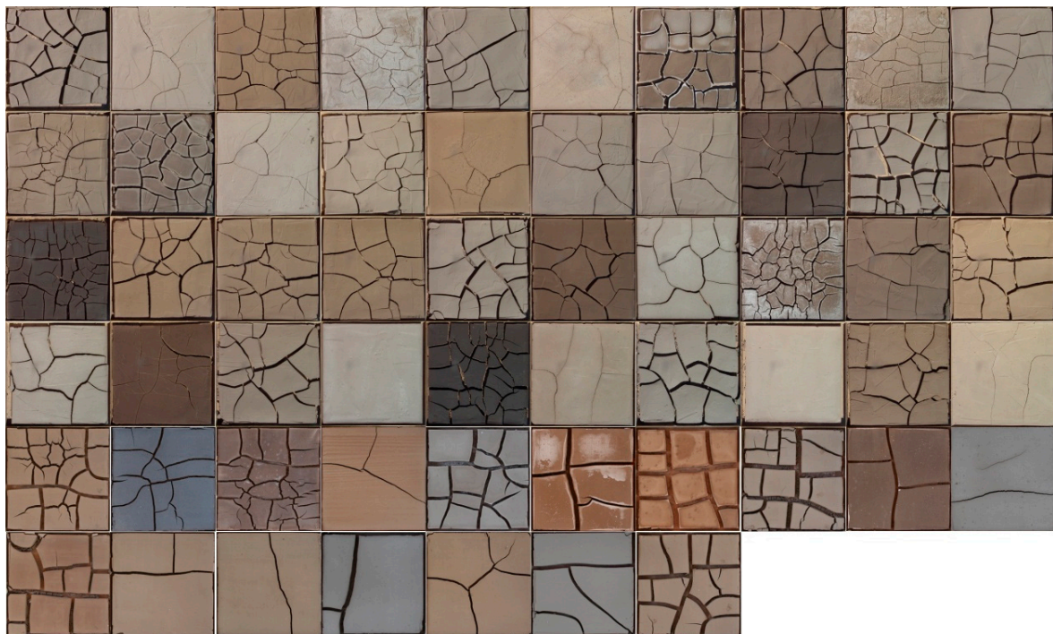
Figure 2. Cracked soil samples after drying process.
