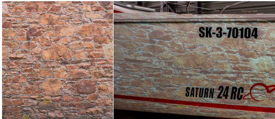
Figure 12. Left—the sample texture used during SfM imaging; right—its projection on the hull.
