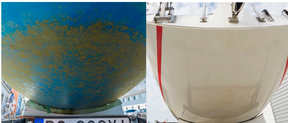
Figure 9. Comparison of the texture of the first sailboat (Saturn 720)—left; and the second one (Saturn 24RC)—right.
