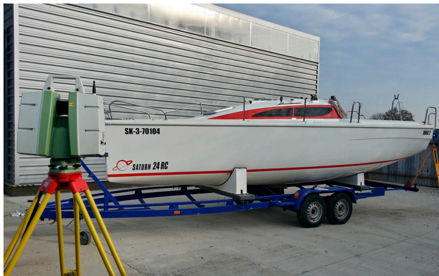
Figure 2. Leica ScanStation C10 at the survey station during orientation to 6 inch high definition surveying (HDS) target.
