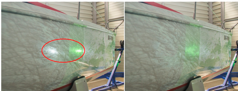
Figure 13. Left—reflections from oblique imaging; right—partial elimination using a polarisation filter.
