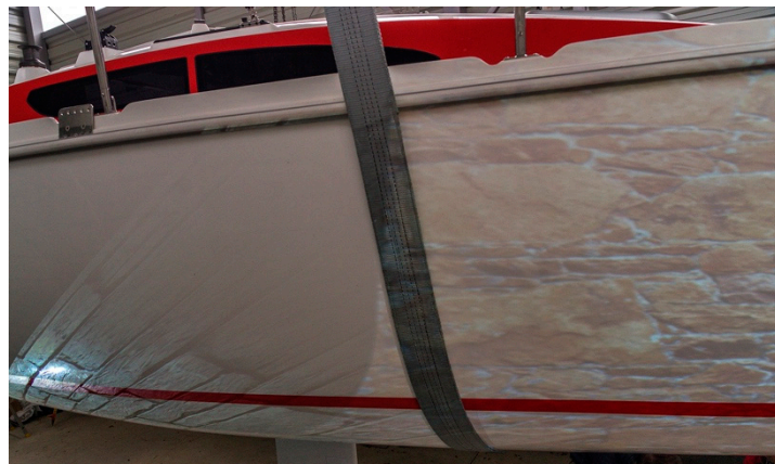
Figure 10. Detail of the suspension system using hanging straps for placing the sailboat to the appropriate height.
