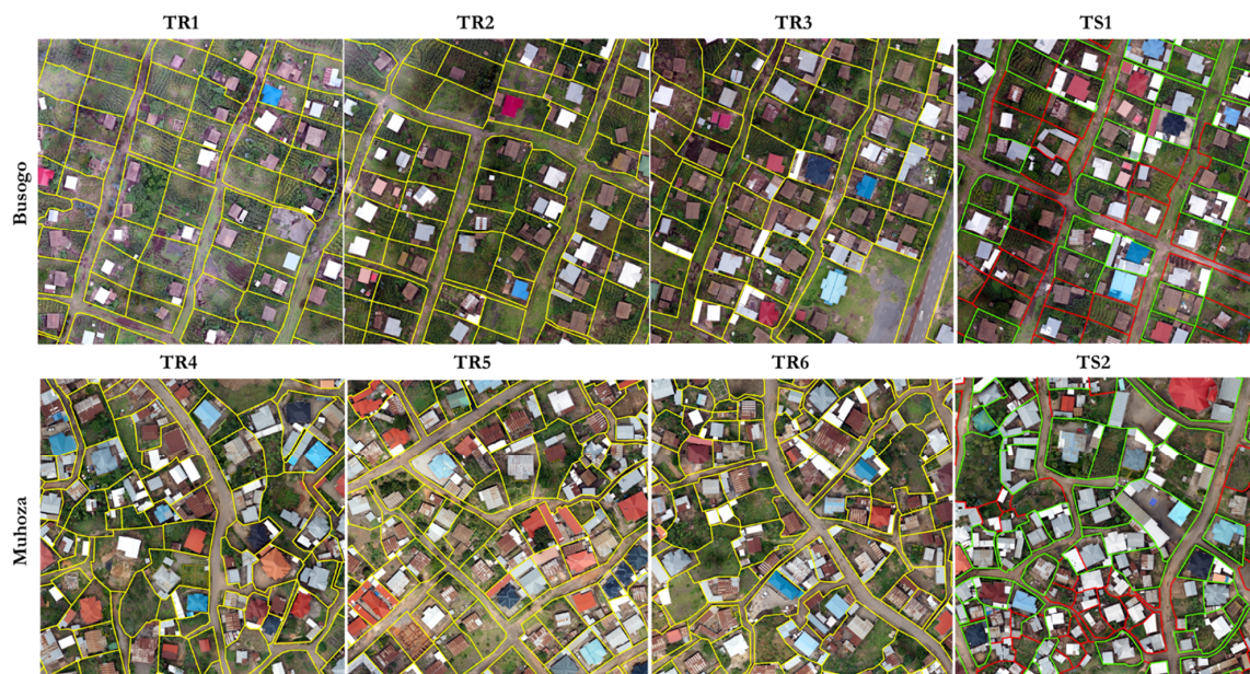
Figure 2. The Unmanned Aerial Vehicle (UAV) images and boundary reference for selected tiles. TR1, TR2, TR3 and TS1 are selected tiles from Busogo; TR4, TR5, TR6 and TS2 are selected tiles from Muhoza. For each area, the former three were used for training and the last one was used for testing the algorithms. The boundary references in TR1~TR6 are the yellow lines. In TS1 and TS2, we separated the boundary references as visible (green lines) and invisible (red lines).
