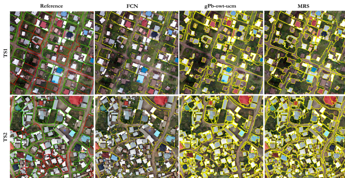
Figure 5. Reference and classification maps obtained by the investigated techniques. The visible boundary references are the green lines; the invisible are the red lines; and the detected boundaries are the yellow lines.
