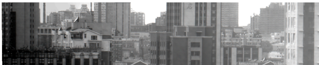
Figure 8. Urban remote sensing panoramic mosaic image with image rotation compensation and image translation compensation under long integral time.
