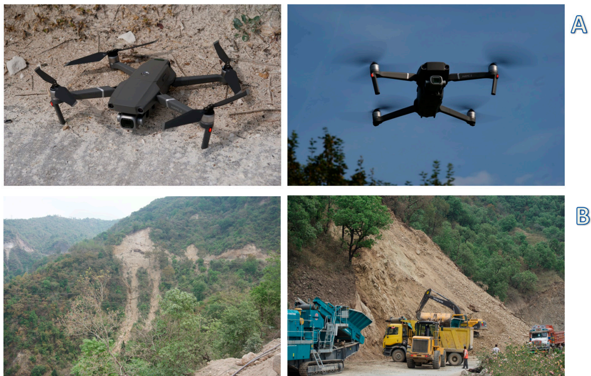
Figure 2. (A) The unmanned aerial vehicle (UAV) used to obtain remote sensing imagery for this study (a DJI Mavic 2 pro), and (B) field photographs of slope failures observed during a field visit to the Himalayas in April 2019.
