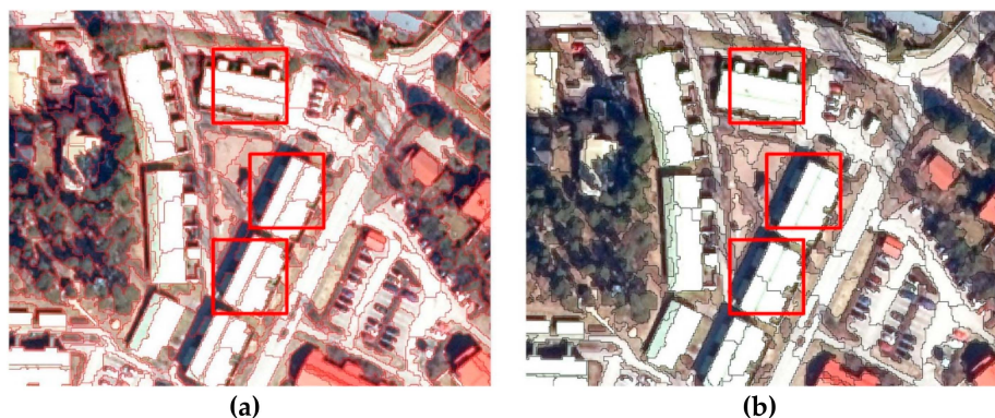
Figure 20. The comparison of point cloud (PC) added and non-added data in segmentation. Red line (a) represents RGB and black line (b) is PC added.
