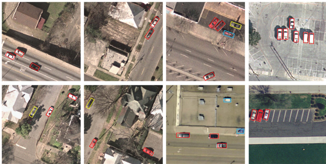
Figure 16. Examples of detection results on the OIRDS [45]. The red boxes (bounding box) denote the truly detected objects, the blue boxes are the false detections and the yellow boxes are the undetected objects.
