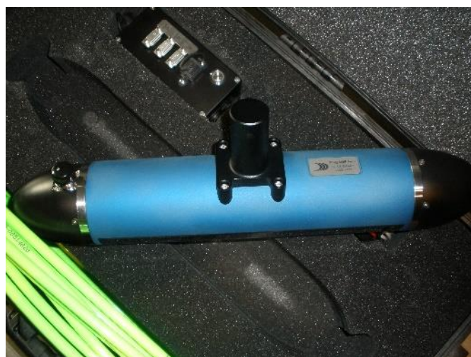
Figure 1. Photograph of the 3D Sidescan 3DSS-DX-450 sonar system (photograph: A. Stateczny).
