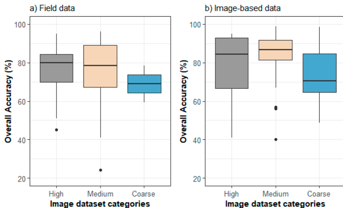
Figure 6. Overall accuracy grouped by the type of image dataset according to spatial resolution used in the classification process, for different types of reference datasets based on (a) field data validation (field plots and GPS) and (b) image-based validation data (single pixels, pixel cluster, and polygons). High refers to less than 10 m pixel size, Medium 10–30 m pixel size, and Coarse refers to images with more than 30 m in pixel size.
