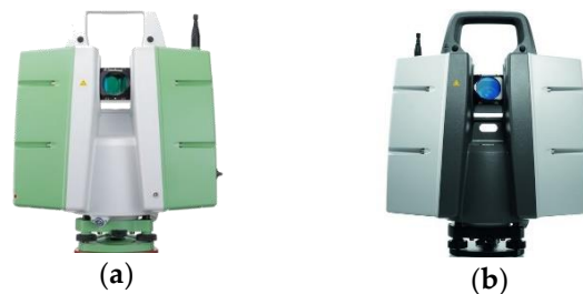
Figure 1. The TLS instruments used in this study: (a) The Leica P20 and (b) the Leica P50. The similarities in chassis, laser beam exit locations, and scanning mechanisms allow for the high registration accuracy of the point-clouds from the two instruments.
