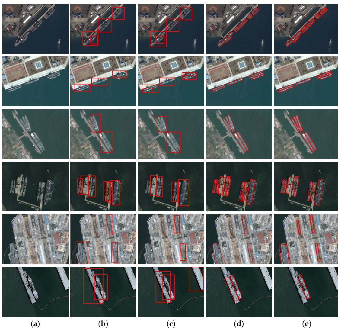
Figure 9. The ship-detection results from different methods. The images from the first row to the fourth row contain many closely docked ships. For the optical remote-sensing images in the last two rows, the backgrounds and the ship objects have very similar textures and appearances. Our method gives accurate detection results for all these cases. (a) Input; (b) Faster R-CNN [9]; (c) SSD [10]; (d) R-DFPN [16]; (e) Ours.
