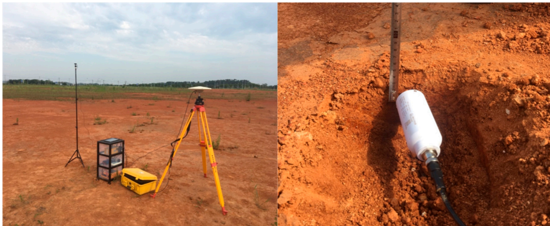
Figure 10. Equipment and surrounding environment (left), soil moisture sensor (right).
