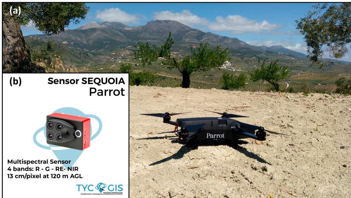
Figure 3. UAV quadcopter (a) and multispectral sensor (b).
