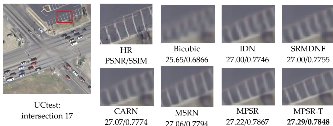
Figure 9. Visual comparison of \times 4 SR results of the UCtest. The best results are in bold.
