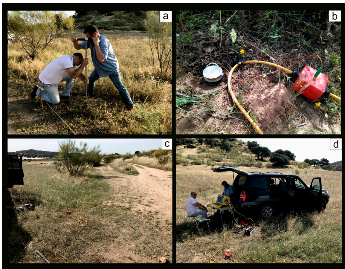
Figure 2. (a) Drilling a hole with an auger to place the non-polarising electrodes. (b) Electrode placed in the ground and connected to the electrical main cable. (c) Profile 1 field layout. (d) Data collection with the resistivity meter.
