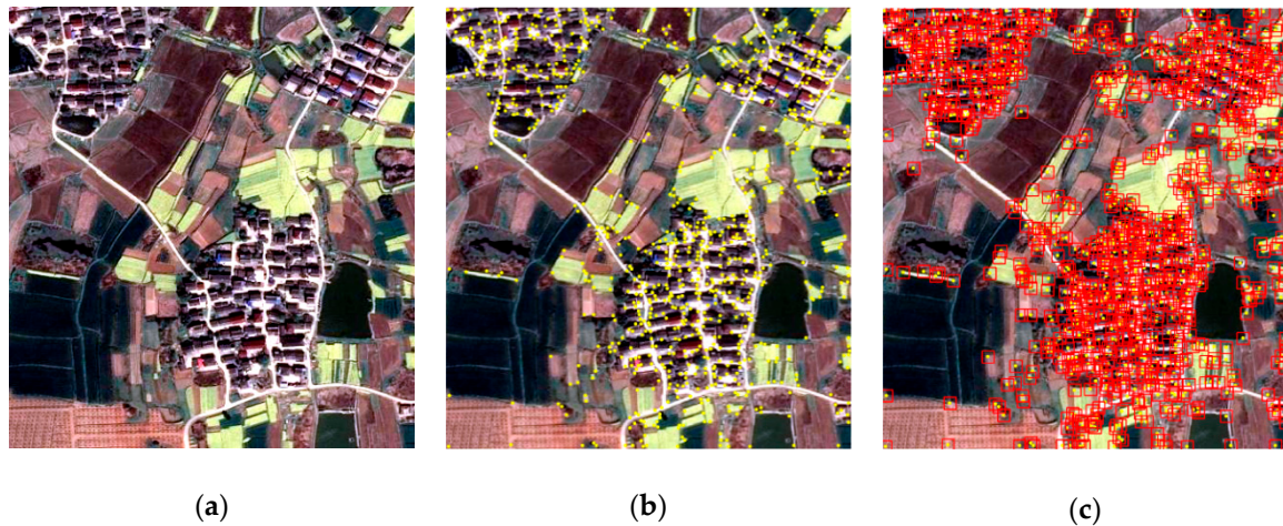
Figure 2. Candidate patches of built-up areas: (a) raw image; (b) detected corners (highlighted with yellow dots); and (c) corner-constrained overlapping image patches (highlighted with red rectangular boxes).
