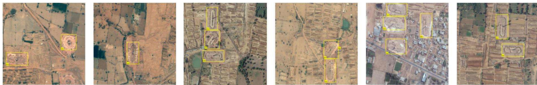
Figure 3. Examples of training samples used in the Faster-RCNN analysis. The yellow rectangles identify kilns in the images. Image data shown from Google Earth provided by Digital Globe.
