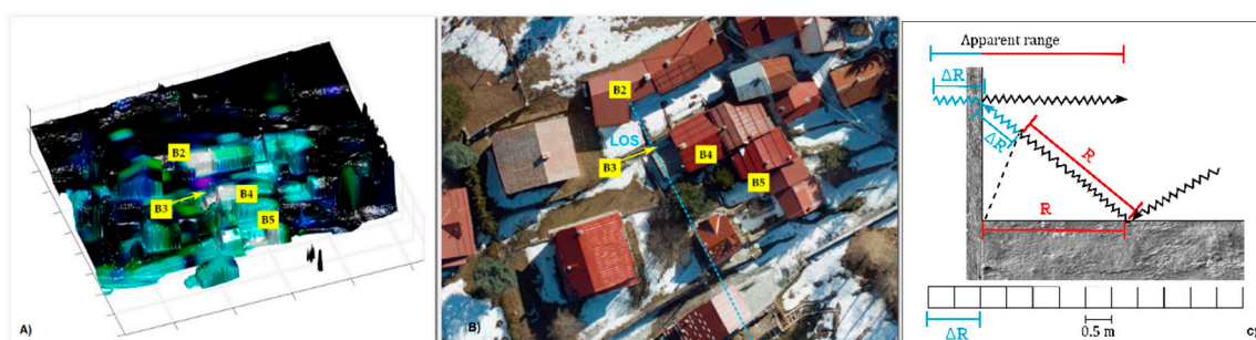
Figure 19. (A) False colour map projected on the DSM; (B) picture of two to four houses with a number label and LOS direction. (C) Scheme of the two scattering modes. The apparent longer range depends on the additional path covered by the radar signal after the first bounce.
