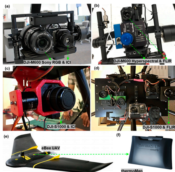
Figure 1. Unmanned Aerial Systems (UAVs) and thermal cameras. Sony RGB and ICI cameras integrated on DJI M600 Pro hexa-copter (a), Headwall hyperspectral and FLIR cameras integrated on DJI M600 Pro hexa-copter (b), DJI S1000 octocopter and ICI camera (c), DJI S1000 octocopter and FLIR & camera array (d), and eBee UAV and thermoMap camera (e,f). Note: eBee UAV and thermoMap camera photos are obtained from this site: https://www.sensefly.com/ .
