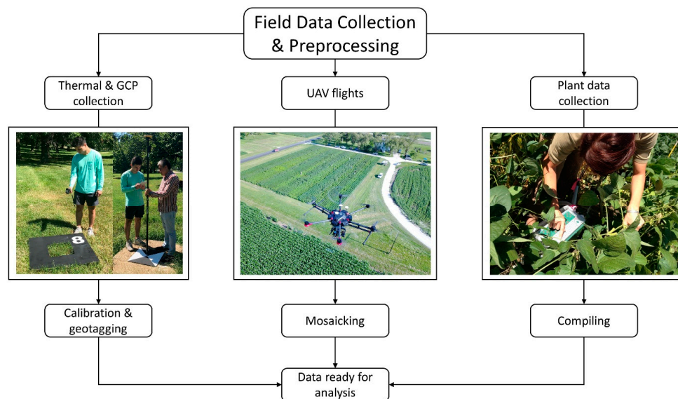
Figure 4. The process for gathering thermal data, UAV imagery, and plant trait data. In the left photo, FLIR TG167 was used to take ground temperature readings over a thermal target, and Trimble Catalyst Differential GPS system was used to record accurate coordinates of ground control targets. In the middle, the UAV system was collecting data over the test site located in Bradford Research Extension Center, Columbia, Missouri. Right photo shows a LI-6400XT Portable Photosynthesis System being used to collect photosynthesis and stomatal conductance.
