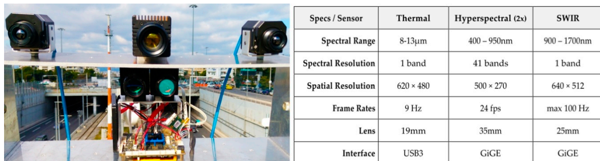
Figure 2. The multisensor system on the left with the thermal (top left and right), the SWIR (middle top) and the two hyperspectral snapshot sensors (middle bottom) on top of the single board computer with the embedded processor. The sensor specifications are presented in the table on the right.
