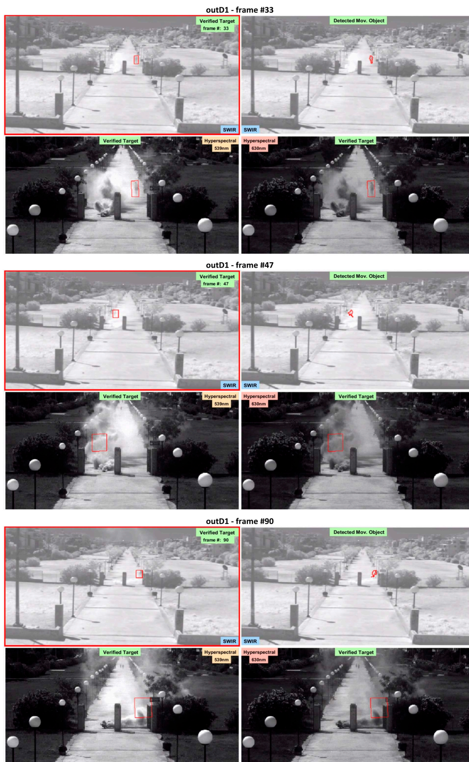
Figure 8. Detection results from the developed method (based on the BS detector) on the outD1 dataset. Frames #33, #47, and #90 are presented along with the intermediate ‘detected moving objects’ and finally ‘verified targets’ overlaid in the SWIR and hyperspectral (539 nm and 630 nm, respectively) bands.
