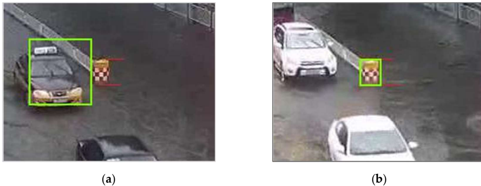
Figure 6. An example of one car being mistakenly recognized as a traffic bucket (a), and an example of the traffic bucket being correctly detected (b) using a relatively large size for the region of interest (RoI). The green box is the bounding box. Due to the low resolution of available video data, these images are not very clear.
