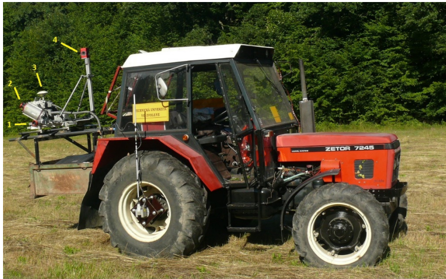
Figure 2. Mobile mapping system RIEGL VMX-250 mounted on tractor Zetor Horal 7245. Two digital cameras (1) and mobile laser scanners VQ-250 (2) are placed on the side of the MMS measuring head. The GNSS antenna (3) is placed on the top of the measuring head and the panoramic camera (4) is placed above the MMS measuring head (Source: Čerňava et al. [20]).
