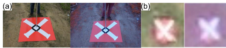
Figure 4. Example of an artificial ground control point (GCP) measuring 100 \times 100 cm: (a) being surveyed with a global navigation satellite system (GNSS) receiver placed in the middle of the marker, (b) aerial image taken by the unmanned aerial vehicle. In the left, RGB representation, and in the right, colour infrared representation.
