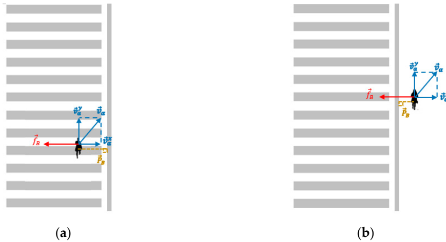
Figure 4. Repulsive and attractive forces at the crosswalk boundary. (a) Repulsive boundary force; (b) attractive boundary force.
