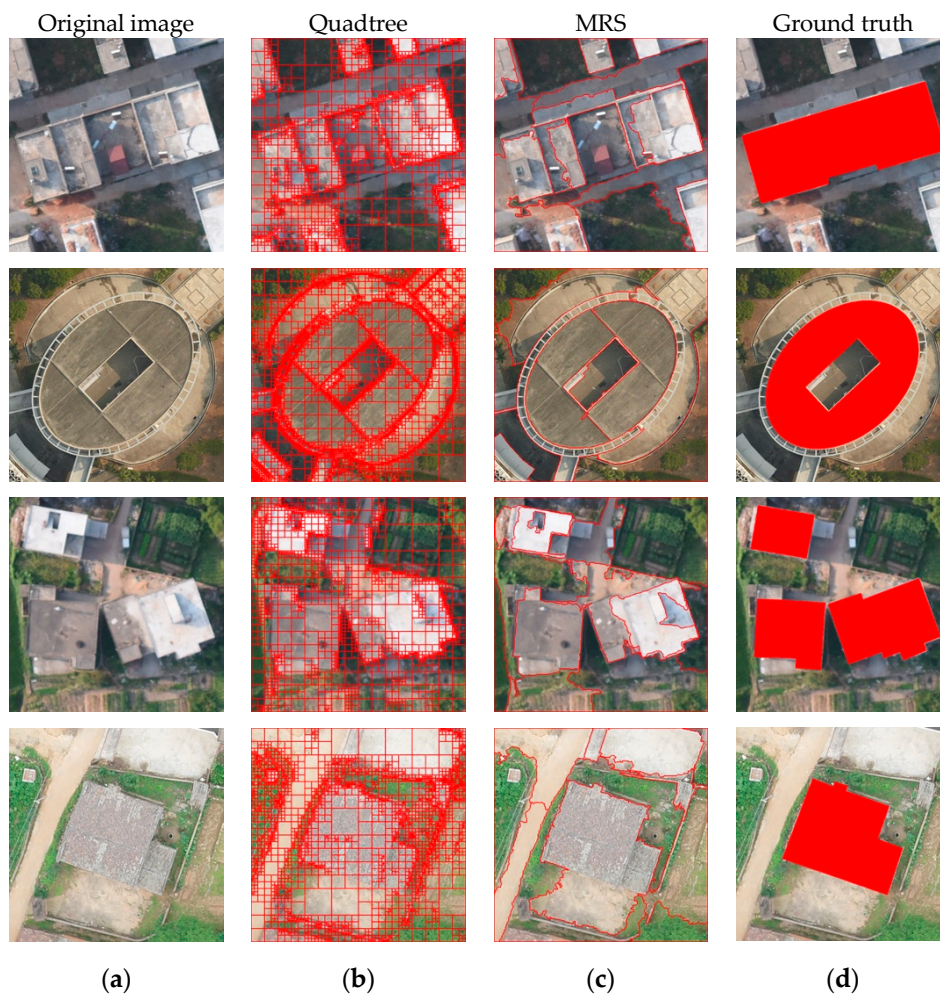
Figure 2. Comparison of building extraction from UAV images using two classical segmentation methods. Column (a) includes four types of buildings in urban and rural areas. Columns (b,c) are the results of quadtree and MRS, respectively; the red lines are the outlines of ground objects. Column (d) is the ground-truth outlines corresponding to (a), with the red regions denoting the buildings.
