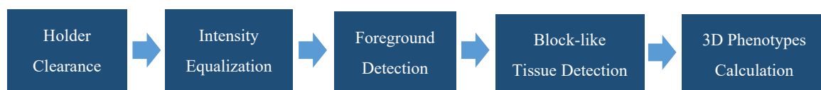
Figure 4. The pipeline of pro-processing of CT image. The parts are all automated.
