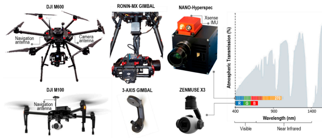
Figure 2. The DJI Matrice 600 and 100 unmanned aerial vehicle (UAV) systems, sensors, and payload used for data collection over the experimental sites. The Headwall Nano-Hyperspec collects surface radiance in the wavelength range from 400–1000 nm across 270 continuous bands. The Zenmuse X3 camera collects RGB radiance in the visible spectral range across a single 400–700 nm spectral range.
