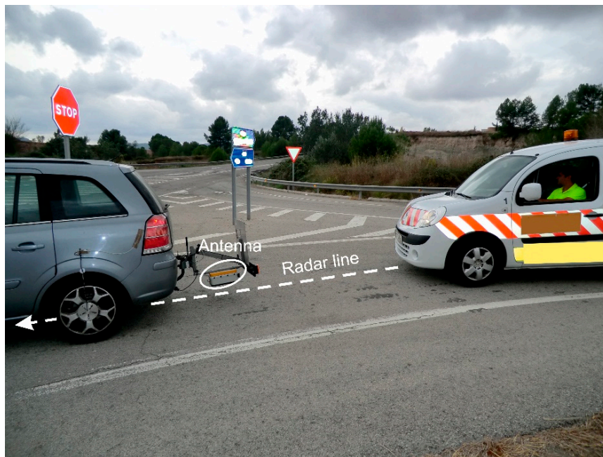
Figure 5. Radar data acquisition with a 900 MHz center frequency antenna.
