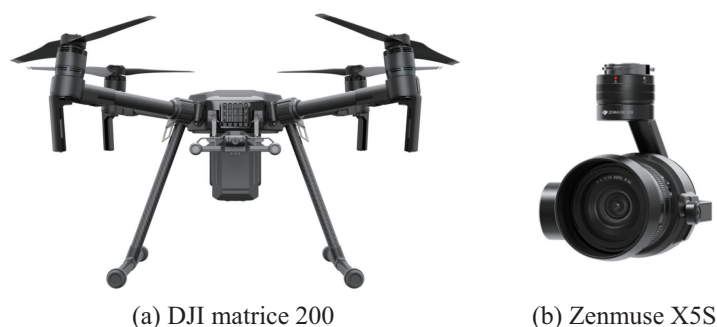
Figure 3. Airborne platform. (a) DJI matrix 200 quadcopter. (b) Zenmuse X5S gimbal and camera.
