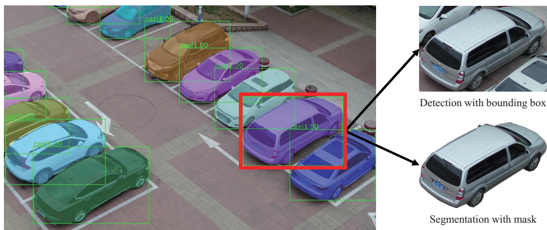
Figure 10. Comparison of our vehicle segmentation and detection. For this vehicle, approximately 38% region in the bounding box is from the background, whereas the region in the mask contains almost no background.
