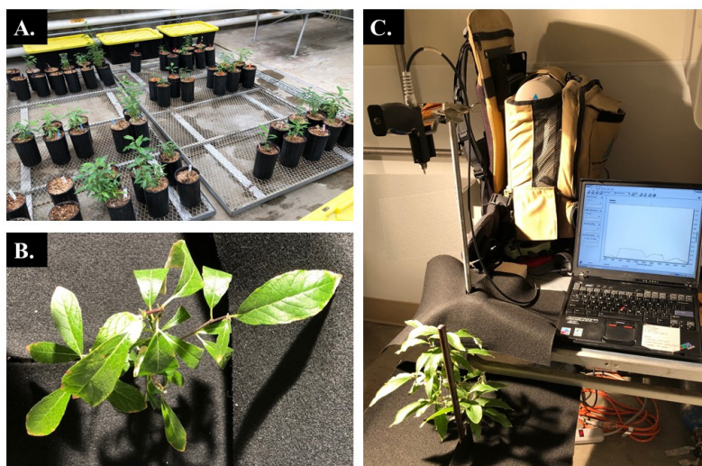
Figure 1. Experimental and data collection set up. Willows were grown in a greenhouse setting (A) and canopy spectra were collected using an FieldSpec Pro Full Range Spectroradiometer (C). A spectrally flat black-foam material below the canopy to avoid introducing soil and background noise (B).
