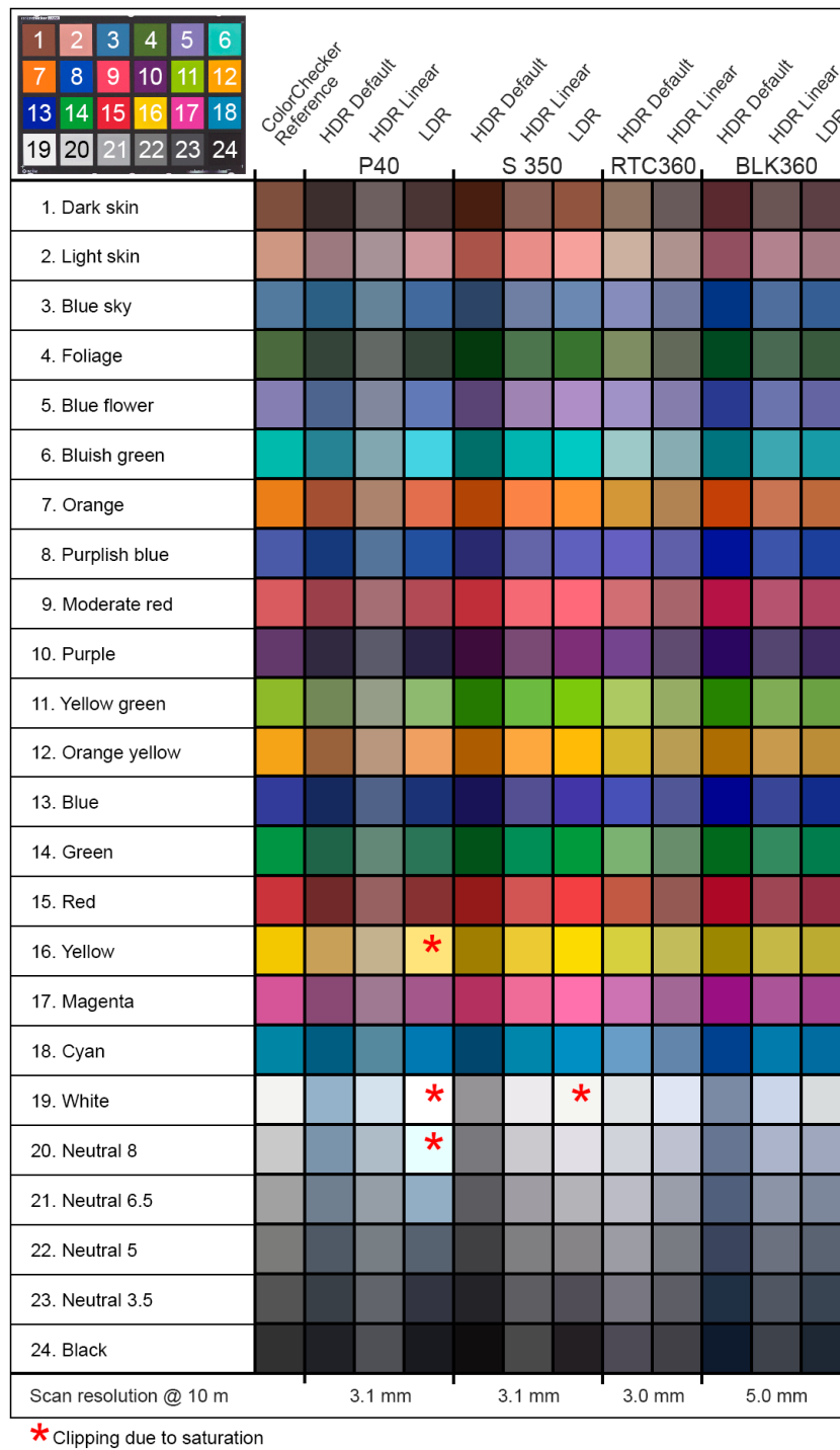
Figure 8. A comparison of the measured colors and the ColorChecker reference colors per patch for each scan with high resolution settings (closest to 3 mm @ 10 m).
