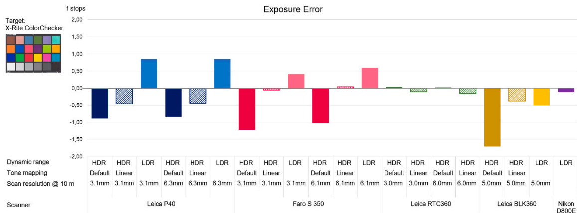
Figure 6. The exposure error of each scan measured from the ColorChecker chart.
