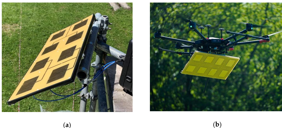
Figure 3. Patch array antenna (a) mounted on tower during sky measurement; (b) mounted on multi-copter drone during flight measurements.
