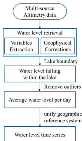
**Figure 2.** Flowchart of the combining multisource altimetry data.
