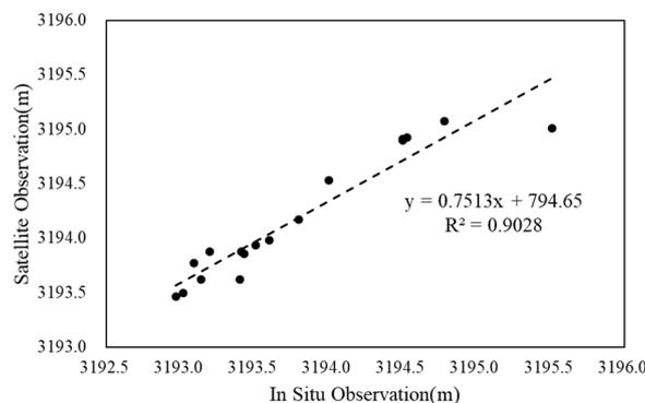
**Figure 3.** Correlation between in-situ water level observations and satellite altimetry observations (from Hydroweb and DAHITI) for Qinghai Lake.
