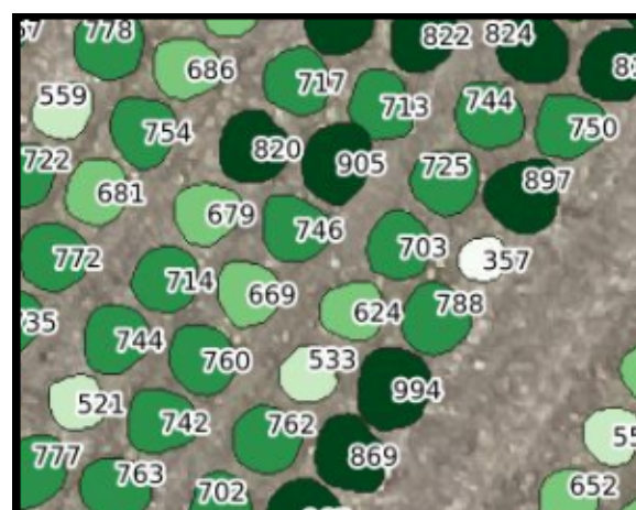
Figure 7. Sizing of each lettuce plant in cm 2 for a sample image patch of L1 field. Each lettuce is overlaid with its predicted mask. The masks' green colour becomes increasingly darker with the plant size.
