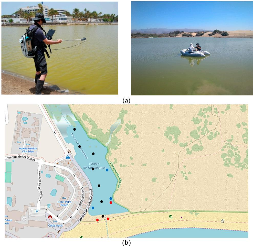
**Figure 3.** (a) Field campaigns to measure surface radiance (left) and water quality and bathymetry (right), and (b) in situ sites monitored in the Maspalomas lagoon ecosystem during the campaigns performed in 2017 (red), 2018 (blue) and 2019 (black).
