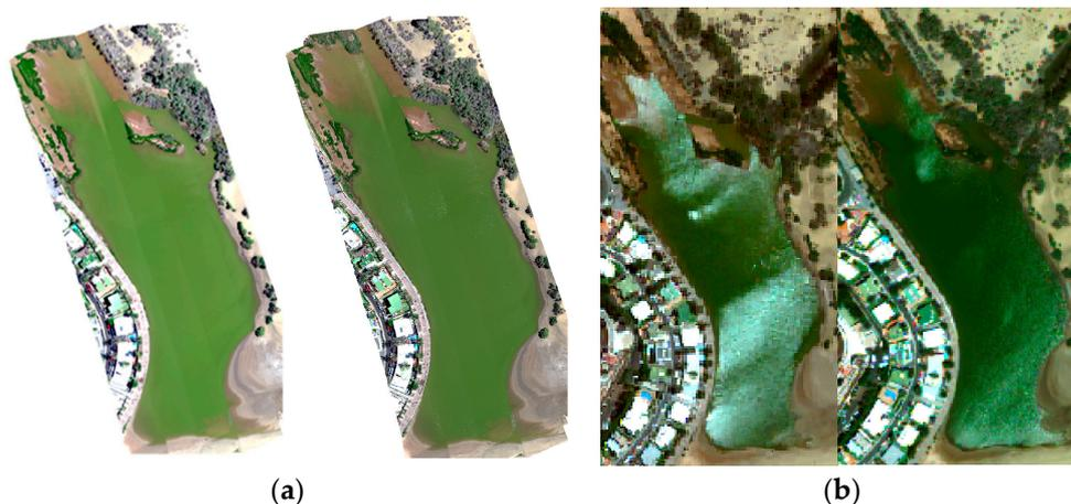
**Figure 10.** Sunlight correction of the Maspalomas inner-lake multiplatform color composite imagery: (a) Pika-L drone imagery and (b) WorldView Satellite.
