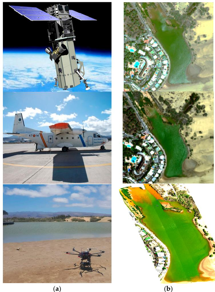
**Figure 2.** (a) Multiplatform Earth observation systems for the monitoring of water quality in the Maspalomas lagoon ecosystem and, (b) true color RGB composite data obtained from Worldview-3 multispectral satellite (31 May 2017), Airborne Hyperspectral Scanner(AHS) hyperspectral airborne (2 June 2017) and PIKA-L sensor aboard drone platform (4 June 2018).
