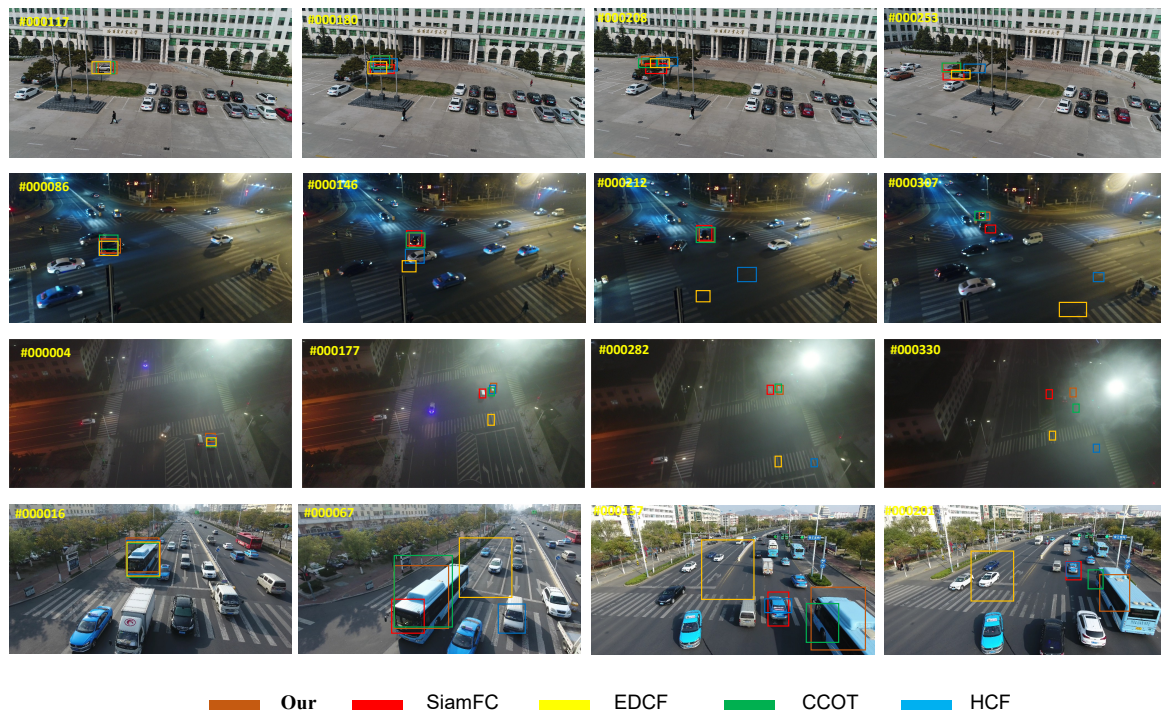
Figure 10. Experimental results of different trackers on challenging sequences (from top–down are S0201 , S0301 , S1306 and S0602 from the UAVDT [7] dataset). The tracking results of SiamFC [20], EDCF [19], CCOT [47], and HCF [37], as well as the proposed algorithm are denoted by different colored bounding boxes.
