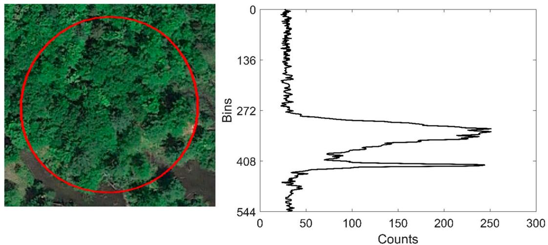
**Figure 4.** Example Geoscience Laser Altimeter System (GLAS) data, ~70 m in diameter ( $44^{\circ}5'10''$  N,  $71^{\circ}17'43''$  W), in 2004. Image in the left panel is from Google Earth<sup>®</sup>, and the right panel is a waveform return where the upper and lower peaks come from the forest canopy and the ground surface, respectively.
