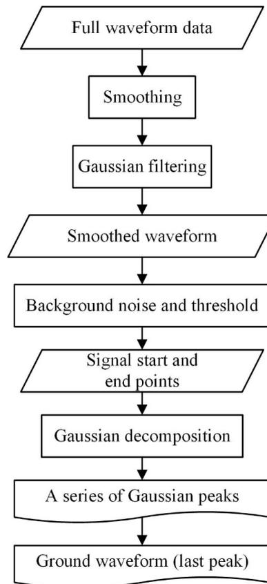
Figure 6. Preprocessing of the full waveform data.
